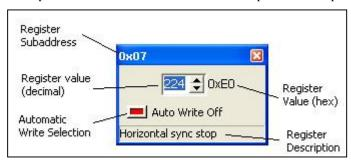
by right clicking the grid and then selecting 'Increment/Decrement Current Register with a Spin Control' from the pop-up menu. The subaddress of the active cell in the grid will be assigned to the Spin Control. The subaddress is shown in the upper left corner. Clicking on the spin control's up or down arrow will cause the value of that cell to be incremented or decremented. If Auto Write On is checked, then the contents of the cell will be transmitted to the device subaddress when it is
