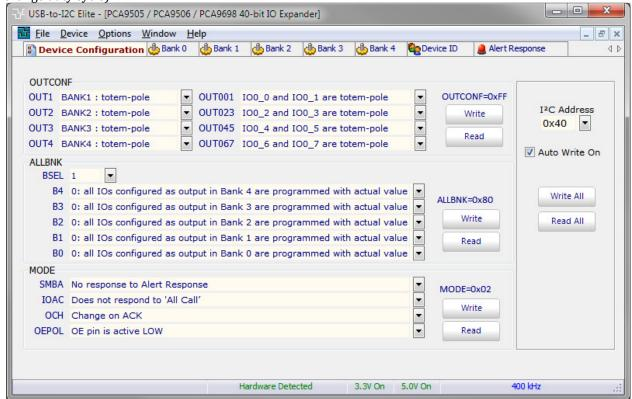
Due to the number of registers in the PCA9698, the application interface is split into multiple pages.
