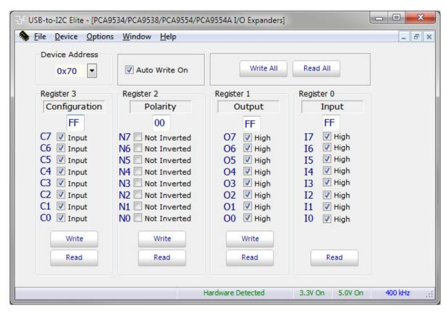
The four devices have four internal registers. All four registers can be read by the bus master while the Input register can only be read.
