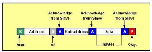
The slave will acknowledge its address after it has been enabled (see Enable Slave paragraph below). The subaddress (or byte address) is a pointer to one of the 256 bytes in the slave data buffer. The I<sup>2</sup>C master will then write any number of bytes to the slave. The byte pointer is incremented after each byte has been written to the slave. The data sent to the slave will wrap back to byte address 0 if it exceeds the maximum size of the slave (see Define Slave Size below).
