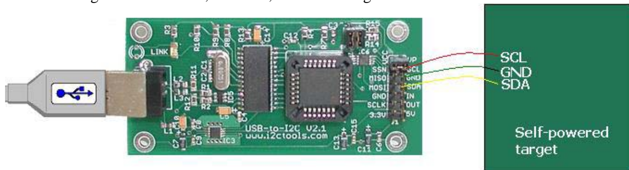
USB-to-I2C Hardware connected to a self-powered target
